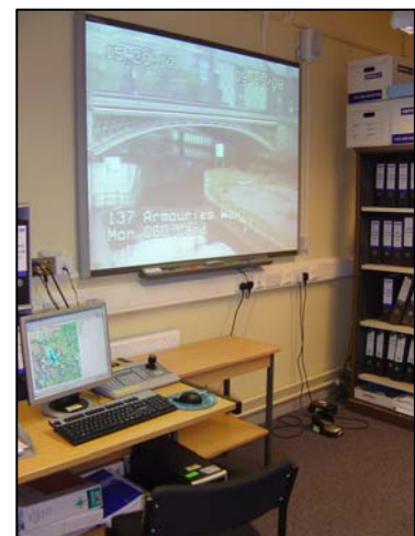
CCTV being used in Land Drainage to monitor water levels on the River Aire
